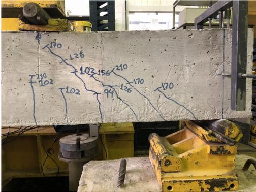
c)  $P = 0,78 \times P_u = 220 \text{ kN}$
