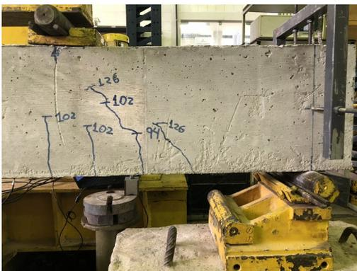
a)  $P = 0,46 \times P_u = 130 \text{ kN}$
