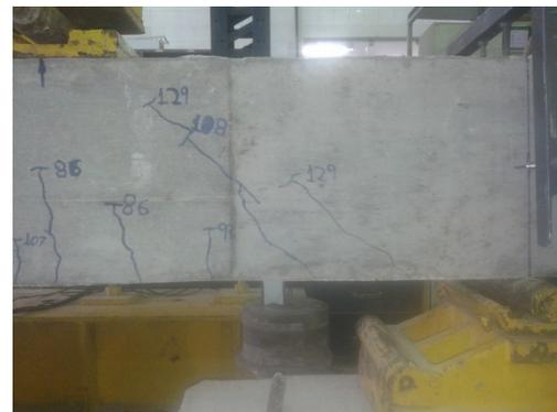
b)  $P = 0,54 \times P_u = 131 \text{ kN}$ .
