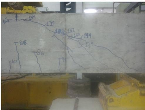
c)  $P = 0,66 \times P_u = 160 \text{ kN}$ .
